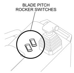
Figure 30. Blade Pitch Rocker Switches
